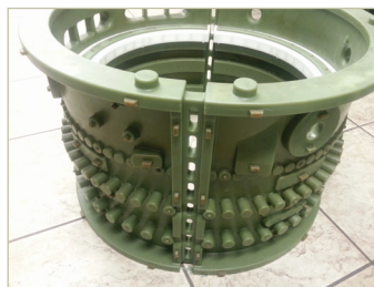
The top image shows the individual pieces of an investment casting mold after machining, which are then assembled into a complete mold (bottom left image). The resulting wax pattern (bottom right image) was used to create a ceramic mold into which molten metal is poured to make the desired part. Note the number of aluminum mold cavities that were machined for this project and the complex details within each. The details are even more evident with the unmolding of the wax pattern.
